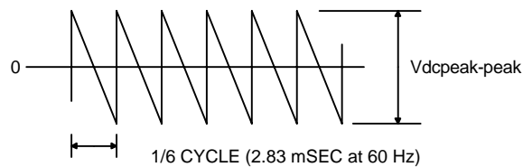
Figure 1 - DSD 412 Output Voltage Waveform with No Motor Rotation (CEMF=0)
