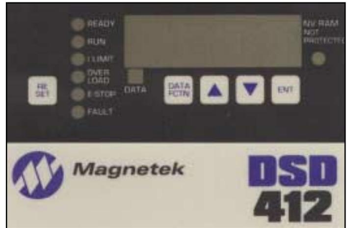
Figure 10: DSD 412 operator interface
