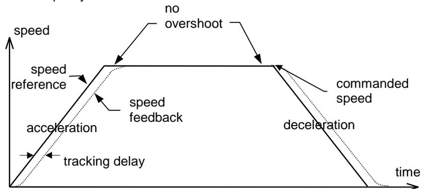
Figure 1 - Elevator Drive Speed Regulator Example
