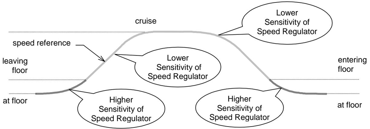
Figure 2 - Speed Regulator Sensitivity Example
